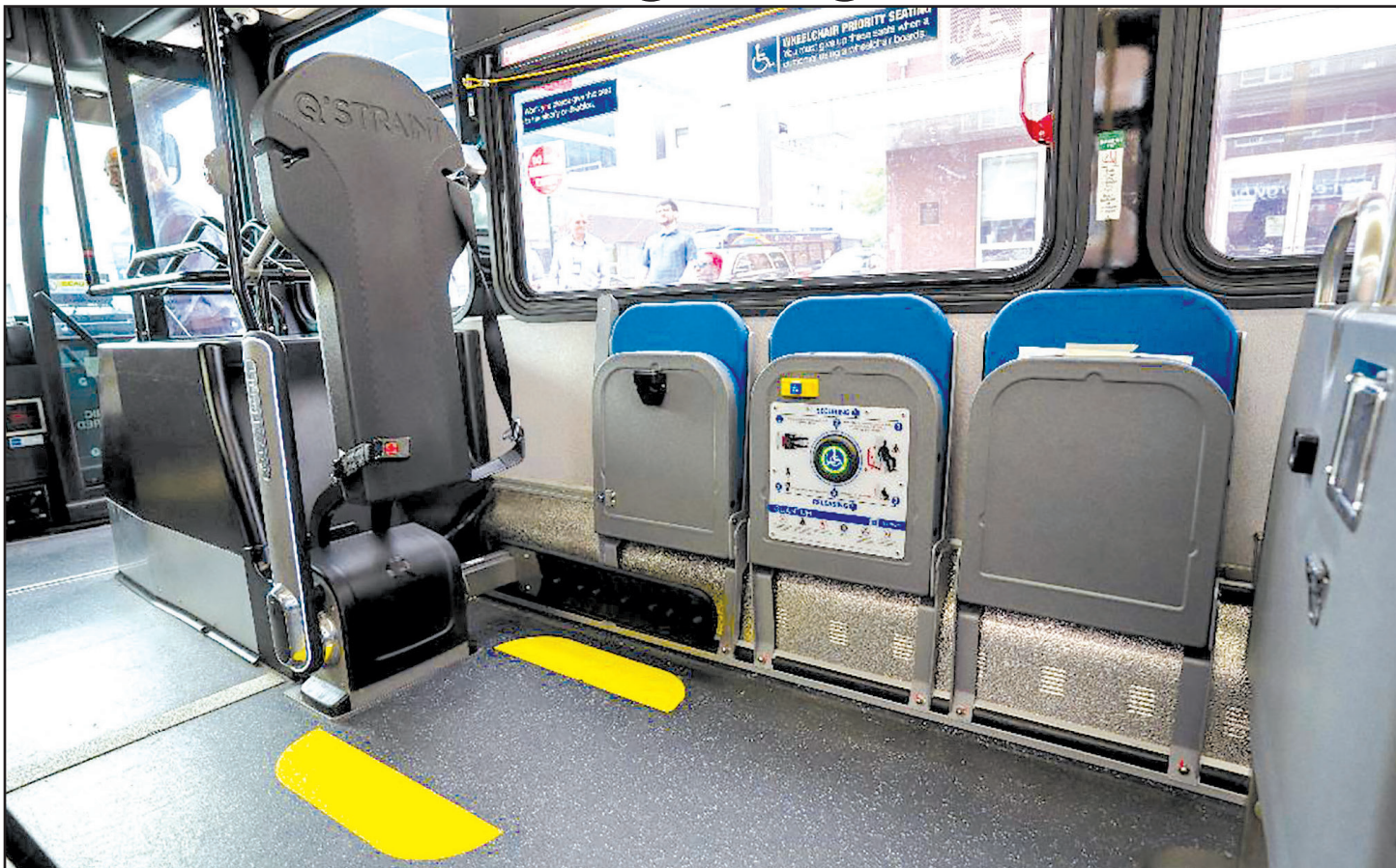
Quantum Self Securement Station is being tested on New York City buses.
